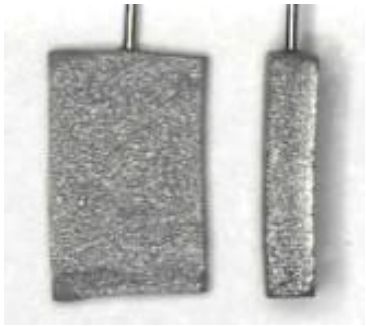
Figure 3. Non-acceptable anode shape post sintering.
