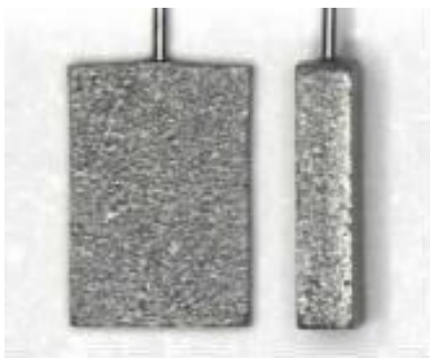
Figure 4. Acceptable anode shape post sintering.
