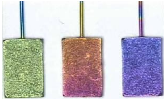
Figure 5. [green] - non-shell formed anode (104 V); [red] - conventionally shell formed anode (125-130 V); [blue] - especially shell formed anode (140 V).
