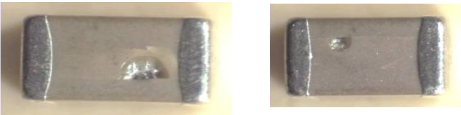
Figure 4. Typical internal voltage breakdown damage on MLCCs
