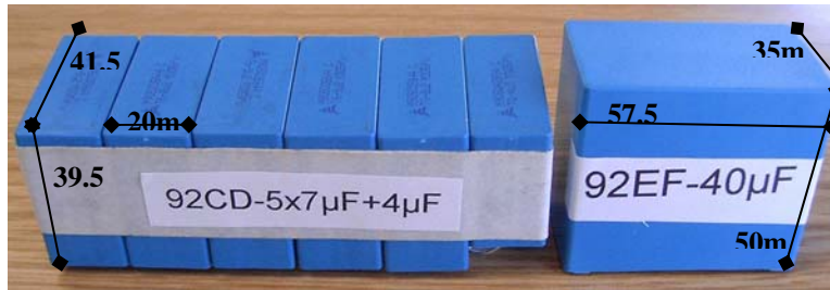
Figure 5: One capacitor of 40\mu\text{F} from new B3292-EF, compared to five capacitors of 7\mu\text{F} and one cap of 4\mu\text{F} in parallel connexion, also 40\mu\text{F} .
