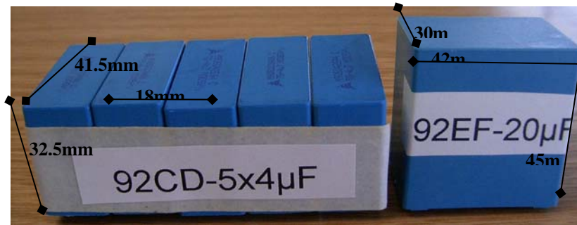
Figure 4: One capacitor of 20\mu\text{F} from new B3292-EF, compared to five capacitors of 4\mu\text{F} connected in parallel, with total capacitance 20\mu\text{F} .
