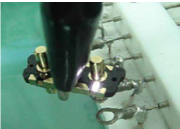
Figure 6. Arc-over on capacitor. The breakdown voltage of the capacitor decrease to 2.5kVdc~3kVdc after mounted inside the connector.
