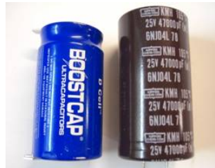
Figure 5: Photograph of a 350 F, 2.5 V, 3.2-cm-diameter electrochemical capacitor (left) and a 0.047 F, 25 V aluminum electrolytic capacitor (right). The devices are approximately the same physical size but the electrochemical capacitor can store ~75 times more energy than the electrolytic capacitor.
