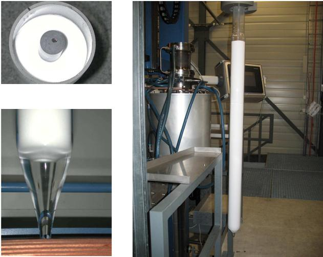
Figure 5. Photographs of sand-clad preforms
