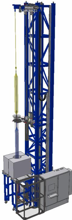
**Figure 3. Conceptual drawing of a sintering system**
