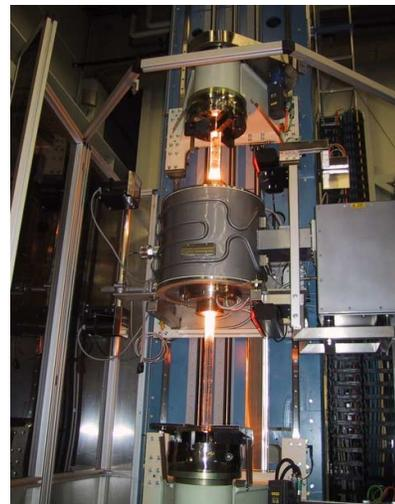
**Figure 4. Photograph of an elongation system**
